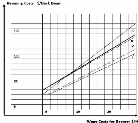
**Fig. 13. Beaming Costs versus Wage Cost (Variants I-V)**
